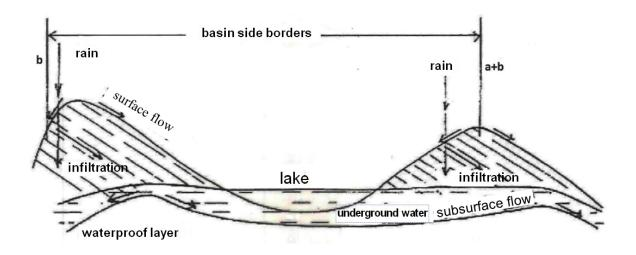
**Figure 4.** Side borders according to the slope of the layer (Suri, 2000): (border a) According to surface flow and (border b) According to subsurface flow
