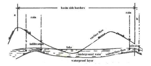
**Figure 3.** Side borders according to the slope of the impermeable layer (Suri, 2000): (border a) According to surface flow and (border b) According to subsurface flow
