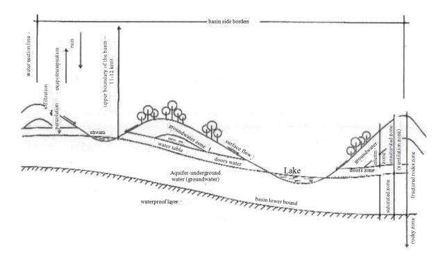
Figure 2. Water movements in the basin and the basin system borders (Suri, 2000)
